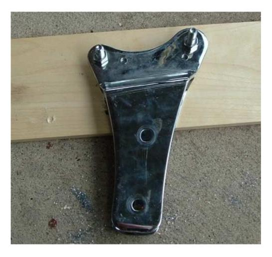
Once that was done, I drilled out the pilot holes so they would accommodate 8mm bolts.
