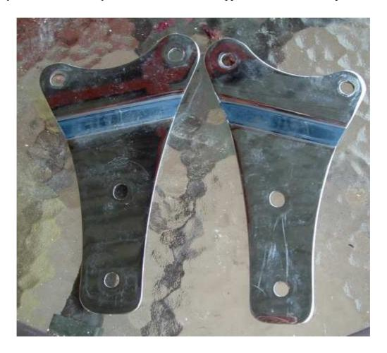
The brackets had these big Mickey Mouse ears that would have to come off as they wouldn't fit behind the arm cover. But first I decided to drill the holes. I lined one out and drilled my pilot holes. Then I bolted the brackets together and drilled through the existing holes so they would be correctly placed on both.
