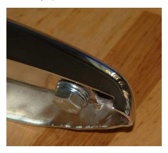
After all the mods, I put a little clearcoat on the brackets where I had cut the ears off to prohibit rusting. Now I got to start putting it on the bike. The brackets went on perfectly and bolted right into place.
